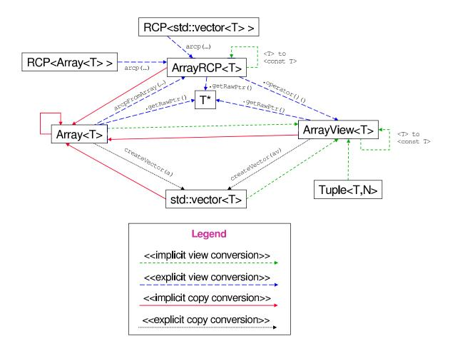
Figure 3. Conversions between array memory management types.
