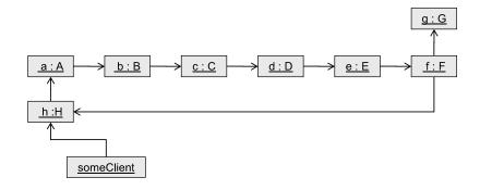
**Figure 10.** Example of a circular chain involving many objects and many classes.
