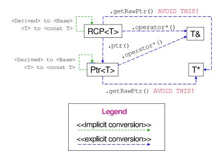
**Figure 2.** Conversions between different single-object memory management types.
