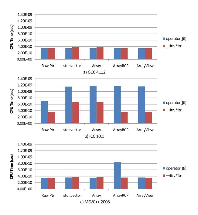
**Figure 14.** Timings for basic Array, ArrayRCP, and ArrayView operations
