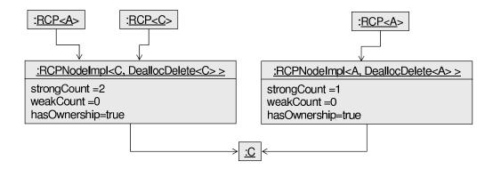
Figure 11. Example of duplicate owning RCPNodeImpl objects
