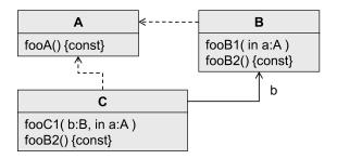
**Figure 1.** UML Class Diagram showing non-persisting and persisting associations for classes in Listing 8 and Listing 9.
