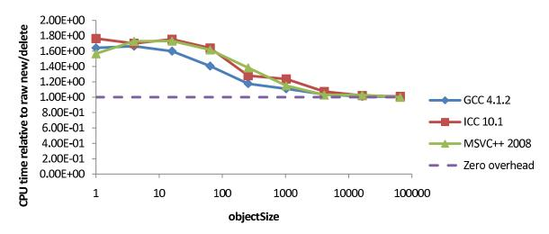
b) Time to dynamically alloc and dealloc std::vector<double>(objectSize) using RCP
